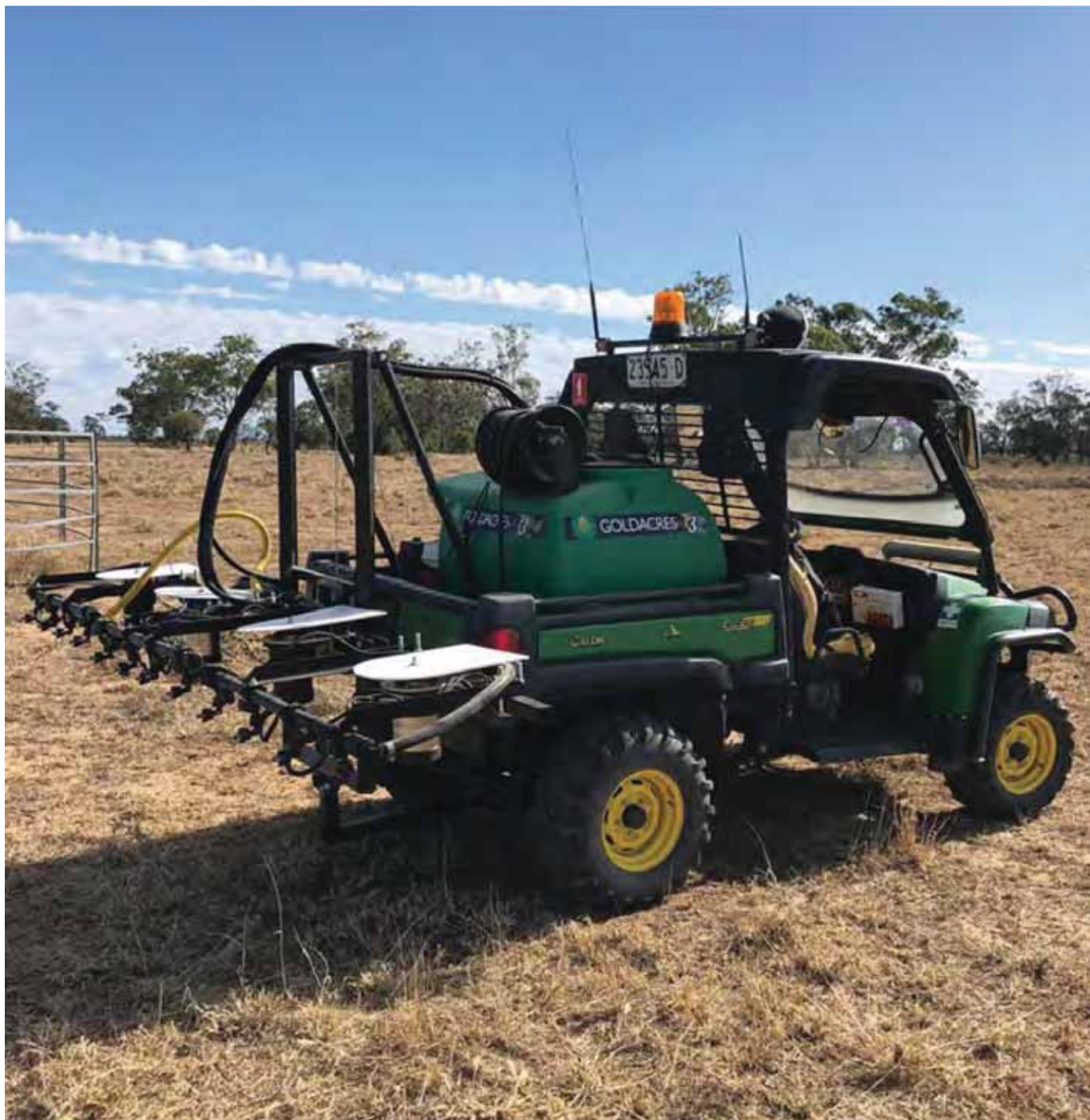
Bilberry recently completed its first Australian commercial-scale trial of green-on-green detection and selective spray.
