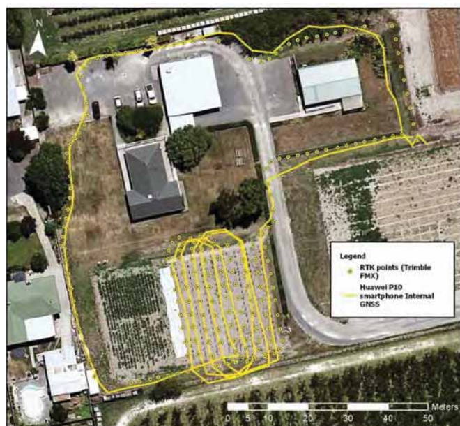
Figure 2. The uncorrected mobile phone trails show inconsistent accuracy when compared to the RTK and inaccuracy of over 1m in places.
