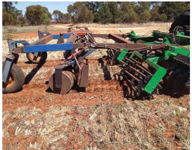
The addition of a roller set at about 45 degrees to the track and a hydraulically adjustable scraper to a commercial track renovator which is used judiciously to reinstate smooth, hard tracks. Photo: M Pfitzner
