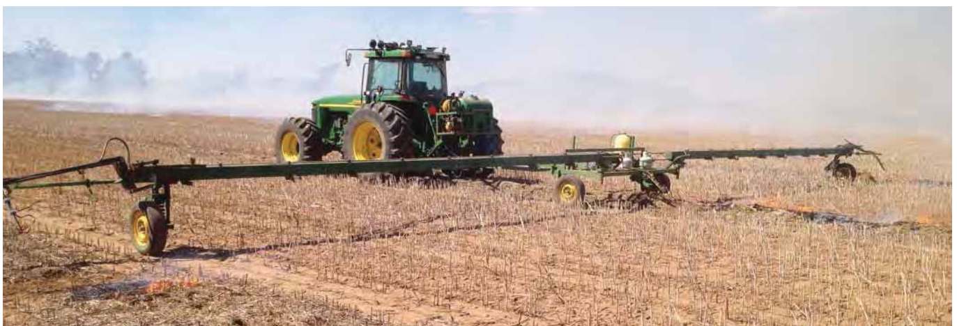
Home-designed and built narrow windrow burner to suit the 12m controlled traffic system. Photo: Emma Leonard
