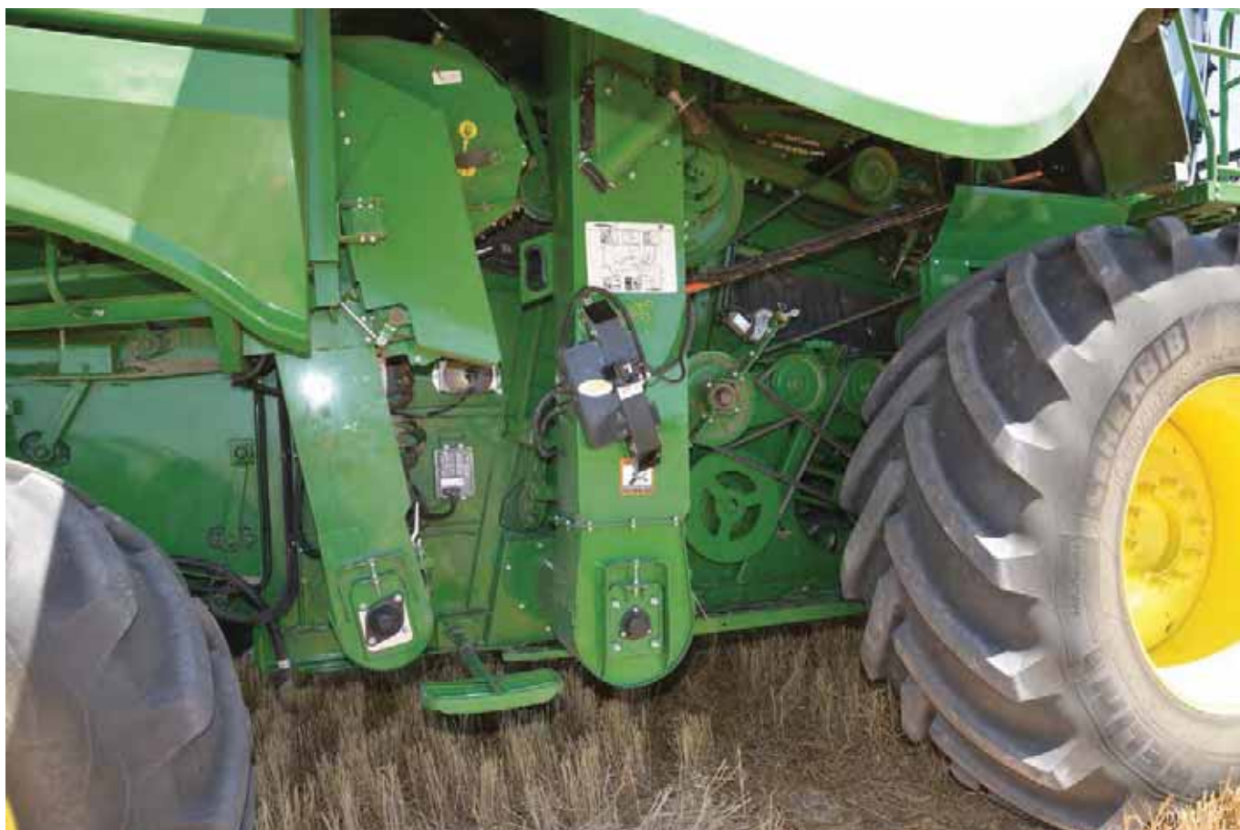
The CropScan is mounted on the clean grain elevator and takes readings approximately every 17m, producing about 15 measurements per hectare. Photo: Emma Leonard
