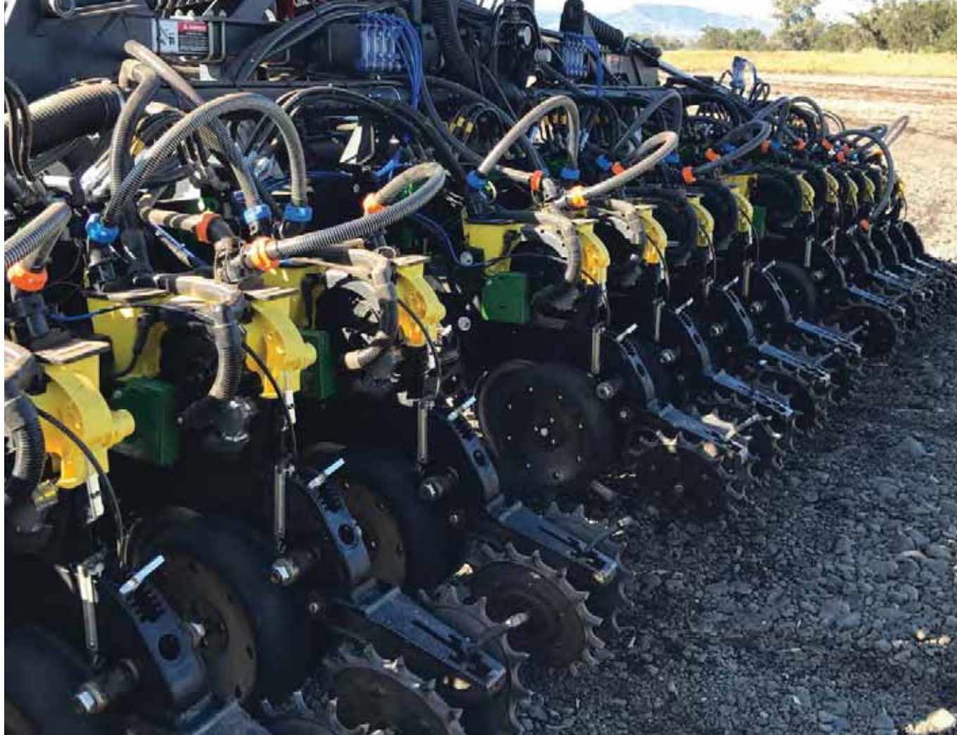
This image shows the V-Set Select, which allows David to plant two varieties side by side. Photo: David McGavin
