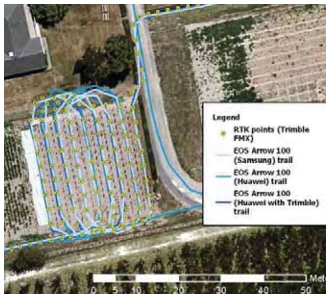
Figure 3. Three successive runs over two days using the Eos Arrow 100 show reliable tracking that compares well with the RTK-GPS plotted points. Deviations are due to the quadbike running different lines rather than GPS errors
