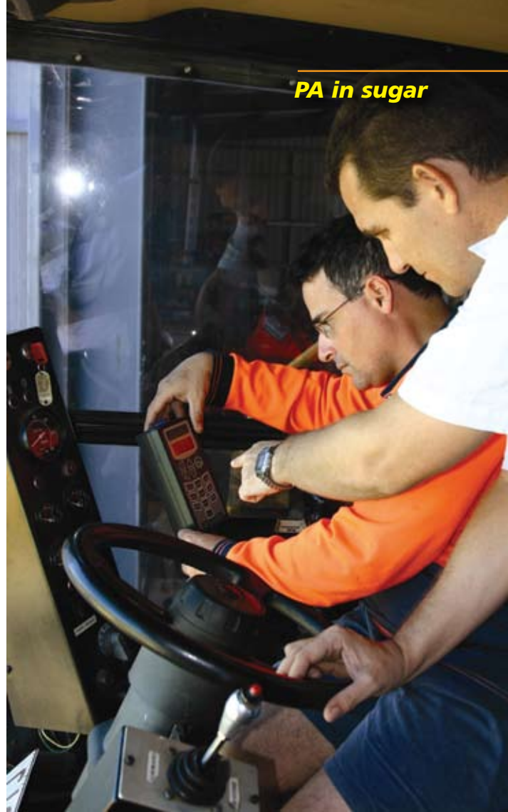
HCPSL Agricultural Systems Information Officer Lawrence Di Bella (L) and Techagro Pacific engineer Angel Luis inspect one of the monitors that will be fitted in the cab of the cane harvesters to track movement and record yield.
